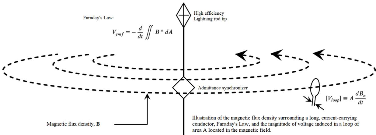
Figure 2: Formulas applied by the high-efficiency lightning rod system according to Faraday's law in a free zone determined by an earthing scalar.
