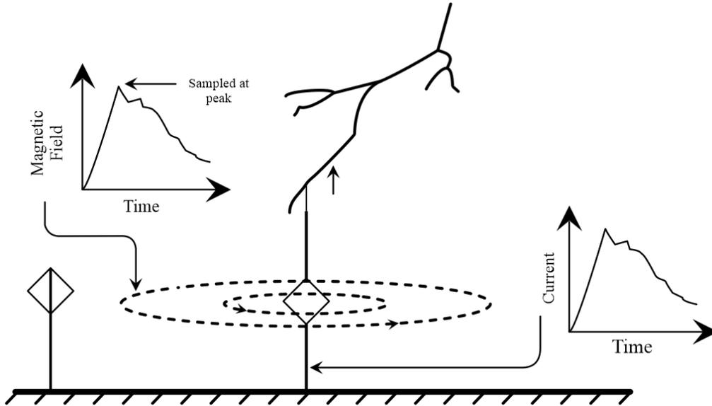
Figure 5: This figure schematically demonstrates the magnetic field values in protection mode and the current value in destruction mode, both based on the time domain, thus demonstrating the great advantage of using a high-efficiency lightning rod system.
